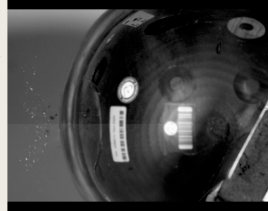
Fig. 7: Screenshots from high-speed camera footage. Shown is the Busch PROtective aramid helmet after impact from a 9mm round.
